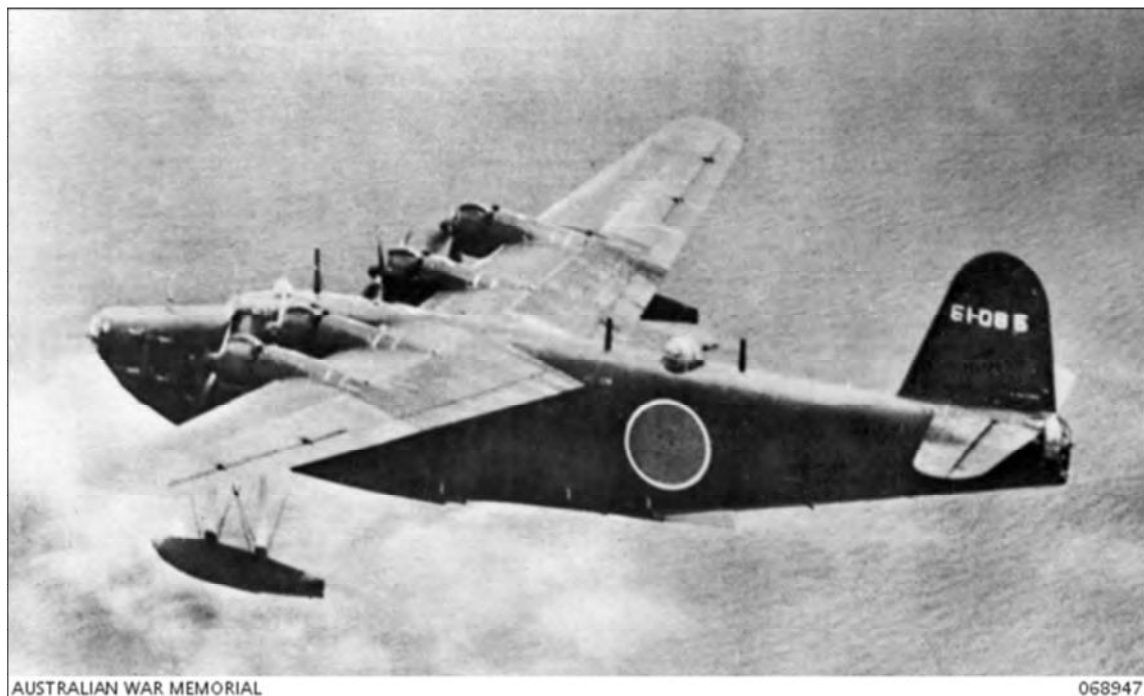
"Emily" four engine bomber reconnaissance flying boat. The Kawanishi navy 2 flying boat, model 12. Japan. Four engine, high wing, all metal monoplane. Power plant: 4 x 1825hp. Mitsubishi "Kasai 22", 14-cylinder motors. Armament: 20 mm cannons and 7.9 mm machine guns. Manufacturers: the Kawanishi Aircraft Co Ltd. (Photograph from Australian War Memorial, 068947 - out of copyright)
