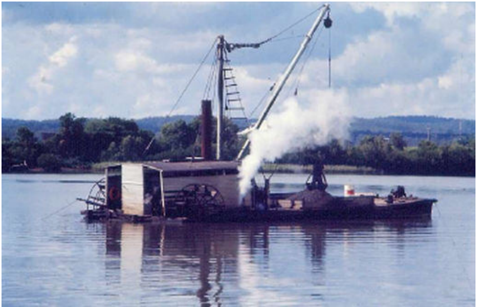
A typical steam paddlewheel drogher on the Clarence River, New South Wales (photo: Greg Jackson)
