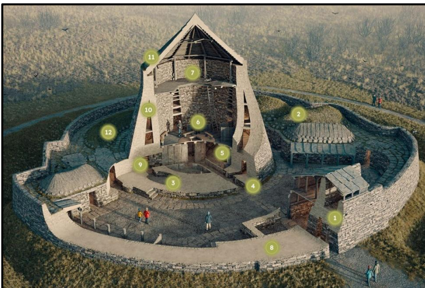
An inside view of Dun Telve, showing the variety of stones used in its construction. The wall is hollow in parts to provide space for the internal staircase.
